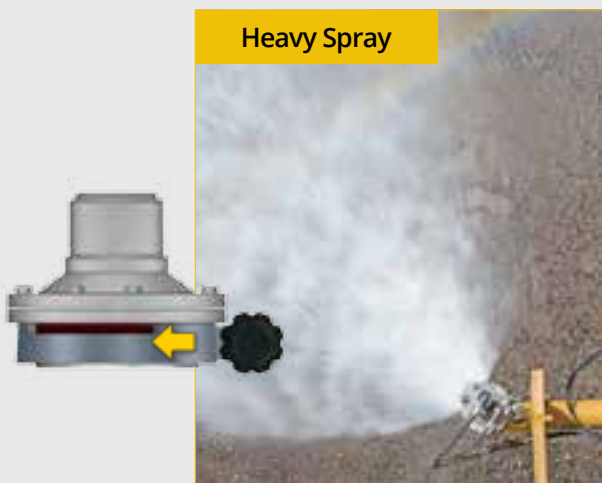
The "heavy" spray head opening is \frac{3}{8} inch tall. This setting provides a very heavy spray of water with reduced width and reach.
