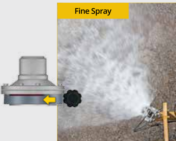
The "fine" spray head opening is \frac{1}{4} inch tall. This setting results in a finer spray of water with maximum reach and width at high pump speeds. This is the recommended setting for most water distribution applications.
