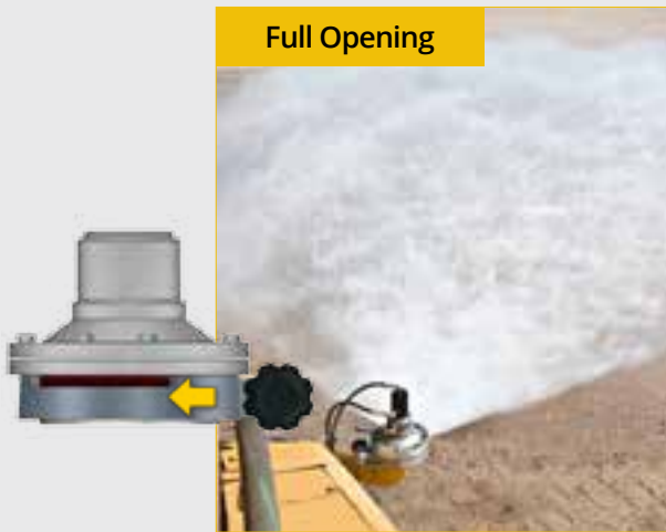
A Mega spray head in the default full (90°) opening setting emits a wide, even fan of fine spray.
