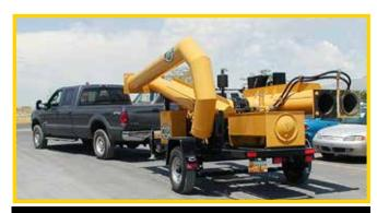
Highway capable chassis. One person operation for travel, set up and use.
