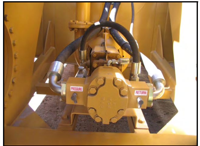
M-4 Water Pump major components and their functions are:
