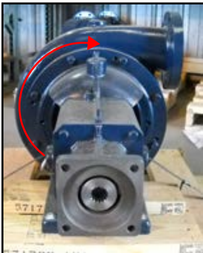
Clockwise rotation as viewed from the drive end of the water pump assembly.
