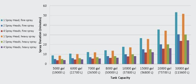
Estimated spray duration for various capacity tanks with four different spray head configurations. Spray duration in minutes is shown on the vertical axis. The "fine spray" opening is ¼ inches in height, and the "heavy spray opening" setting is % inches in height. These flow rates were recorded on an MST8 CAT621K with an M-4B Mega water pump.
