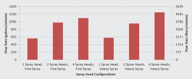
Total flow rates of different spray head configurations. The approximate total flow rates in gallons/minute (left vertical axis) and liters/minute (right vertical axis) of four possible spray head configurations. The "fine spray" opening is ¼ inches in height, and the "heavy spray opening" setting is ¾ inches in height. These flow rates were recorded on an MST8 CAT621K with an M-4B Mega water pump.
