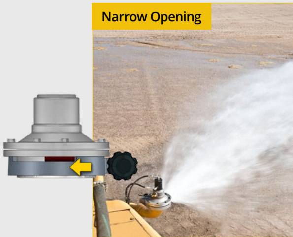
A Mega spray head adjusted to a narrower opening width sprays a more focused stream of water that travels further.
