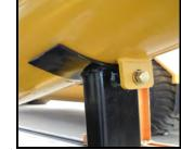
8. Inspect fenders for security and damage.
