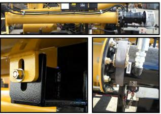
13. Inspect hinge pins, flanges gaskets for lubrication, security, wear and damage.
