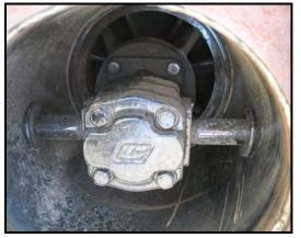
The hydraulic drive motor is coupled to the water pump drive shaft inside the water pump. The drive motor is controlled by the hydraulic control valve, water pump spool. When the lever is moved to the ON position the fluid is directed to the drive motor causing the water pump impeller to rotate, moving water up the inlet boom.
