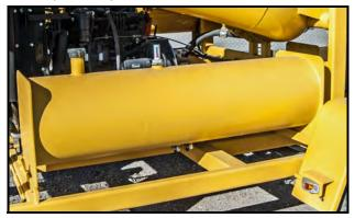
12. Inspect inlet boom, travel locks and mounting for lubrication, security, damage and serviceability.
