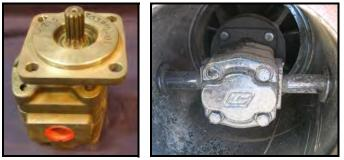
A gear-type hydraulic motor mounted inside the water pump assembly. The hydraulic motor receives hydraulic oil flow from the hydraulic system controlled by the hydraulic control valve at 1,900 - 2,800 PSI (13,000 - 19,300 kpa) and flow rates up to 35 GPM (135 lpm) for operation. The hydraulic motor is coupled directly to the water pump shaft and rotates
