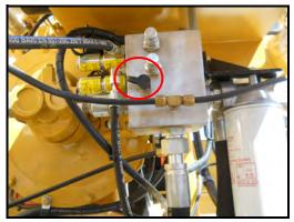
3. With the engine operating at high idle, operate the PUMP UP switch and observe the reading on the pressure gauge.
