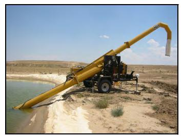
The MMP4 needs a minimum of 2.5 feet (0.76 meters) of water above the inlet of the water pump for proper operation.
