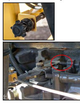
18. Ensure the newly installed throttle cable allows engine throttle to fully contact the HIGH idle stop.
