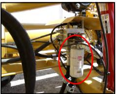
The spin on hydraulic oil filter is in the return to tank hydraulic circuit. All hydraulic oil passing through the system passes through the filter prior to the hydraulic oil cooler. The filter is rated at 400 psi (2,758 kpa). The filter is rated at 10 microns and the filter housing has a built in bypass valve to bypass the filter element when the inlet pressure is too high or the filter becomes restricted.
