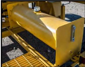
The hydraulic system of the MMP4 consists of an engine mounted hydraulic pump, 35 gallon (135 liter) hydraulic oil tank equipped with an inlet screen, return oil filter, external shut off valve, oil level sight glass and a breather equipped filler cap. The balance of the hydraulic system is designed with:
