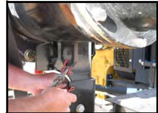
26. Locate and secure the 2 flange bolt assemblies.
