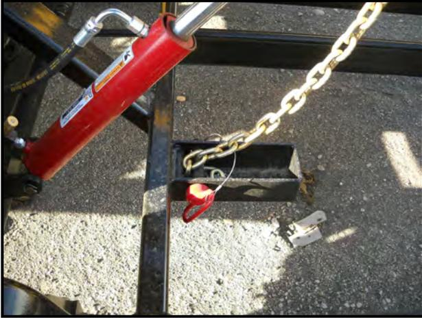
41. Ensure the safety chain is tight, the safety chain shear pin is fully seated and the safety keeper pin is installed.
