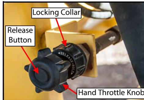
10. Observe the water filling the tank, when the tanker is filled to the desired level, return the MMP4 to LOW idle by depressing the release button on the hand throttle and pushing the knob IN until the engine is at low idle.
