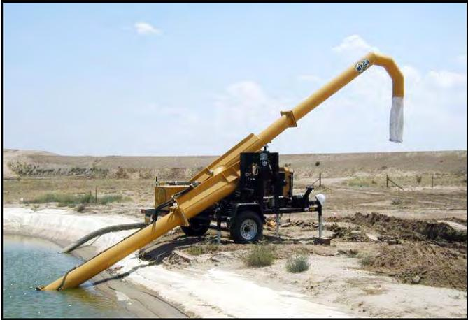
The MMP4 is designed to be towed behind a typical ¾ ton or 1 ton capacity pickup truck. The MMP4 can be transported over the road to just about any water holding pond area used for filling water distribution equipment. The MMP4 can be set up, made ready for operation, and reconfigured for transport by 1 person using simple hand tools.
