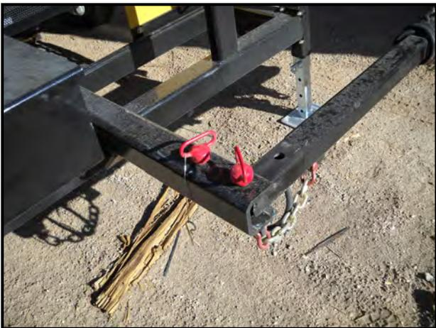
23. Ensure the safety chain on the inlet boom cylinder is tight, the shear pin is fully seated and the safety pin is in place.
