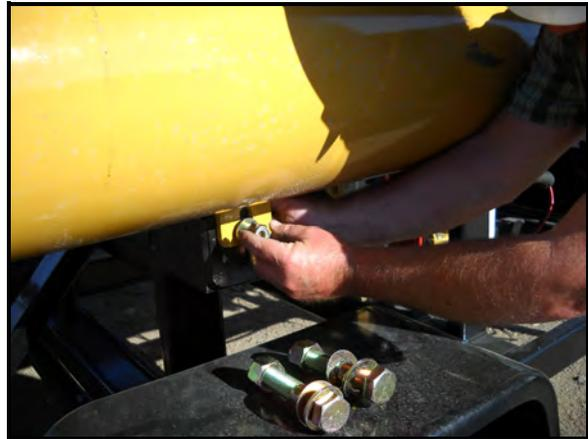
25. Remove the safety strap and the safety chain from the water pump.
