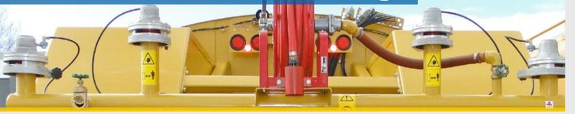
The manual pneumatic spray system is a simpler, cost-effective alternative to the electro-pneumatic spray system, and is available for use on any 24 volt truck with a reliable air supply. The manual pneumatic system can be configured for either an electric or hydraulic water cannon, and comes with a separate tractor air supply protection valve, air-pressure regulator, and manual shut-off valve.
