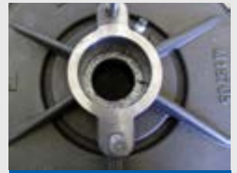
New rope packing installed
