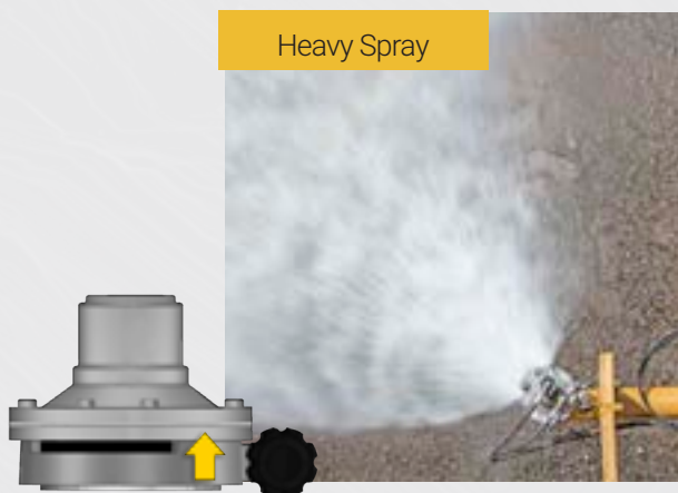
The "heavy" spray head opening is 3/8 inch tall. This setting provides a very heavy spray of water with reduced width and reach.
